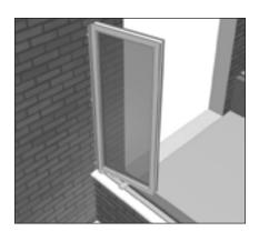
Lift the window and rest onto the support blocks. Pivot the window slightly and slide towards the Wallplate.
