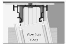
Manoeuvre the window so that the leg on the window frame engages with the hook on the wallplate leg along its entire length.
