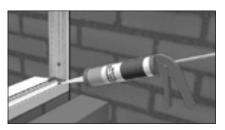
Prior to installing the starter windows, seal the Wallplate to the Cill using the Low Modulus Neutral Cure Silicone.
