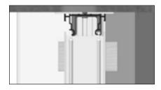
Remove the two packers and firmly push or tap the window downwards to engage the Cill Blocks into the Cill. The base of the window should now sit onto the Cill.
