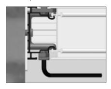
Fit the remaining Quarter Turn Buttons (C117) into the Wallplate (internally & externally) as previously described.
