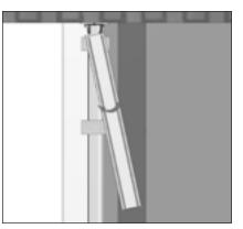
Pivot the window back, so that the inside faces of the Window and Cill are parallel. Check that the opposite hook has fully engaged.
